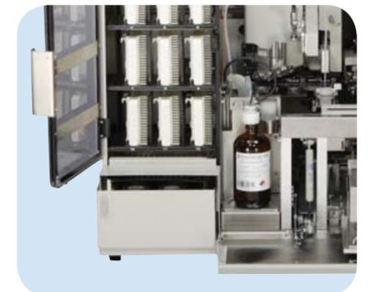
Unloading capacity up to 240 slides, decreased drying time due to use of separate drying racks and air fan.
